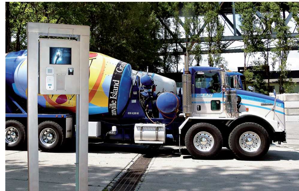
Customer-specific, height-adjustable kiosk terminals for outdoor use for weighing complete trucks and passenger cars including cargo.
