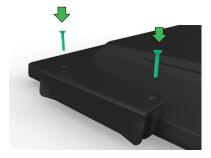
Install the 2 flat head screws included with the kit.
