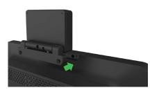
Gently press the NFC Reader into the peripheral bay making sure the connector is mated.
