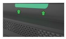
Remove the selected peripheral cover from the display head to expose the peripheral bay.
