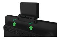
Install the 2 flat head screws included with the kit.
