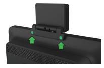
Remove the protective film from the included mylar covers and place the covers over the screws.
