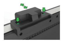
Adjust the forward/back position of the webcam by loosening the two highlighted screws with the included 3mm allen wrench and sliding the webcam head forward as needed. Tighten screws when done.
