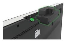
Gently insert the webcam into the peripheral bay taking care to ensure the connector mates properly.
