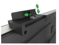
Adjust the tilt angle of the webcam by loosening the highlighted screw and lifting up on the back of the webcam head. Tighten screw when done.
